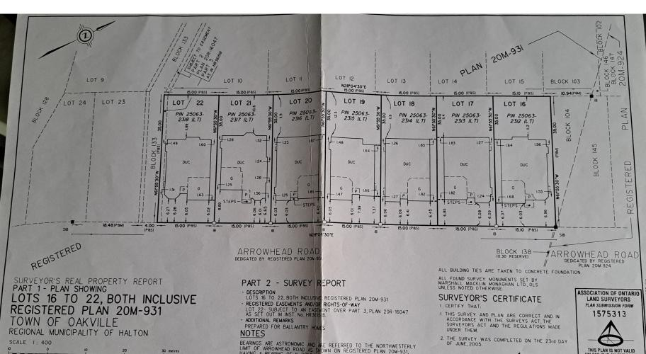
BEARINGS ARE ASTRONOMIC AND ARE REFERRED TO THE NORTHWESTERLY LIMIT OF ARROWHEAD ROAD AS SHOWN ON REGISTERED PLAN 20M-931, HAVING A BEARING OF N 28"04" 10" E.
