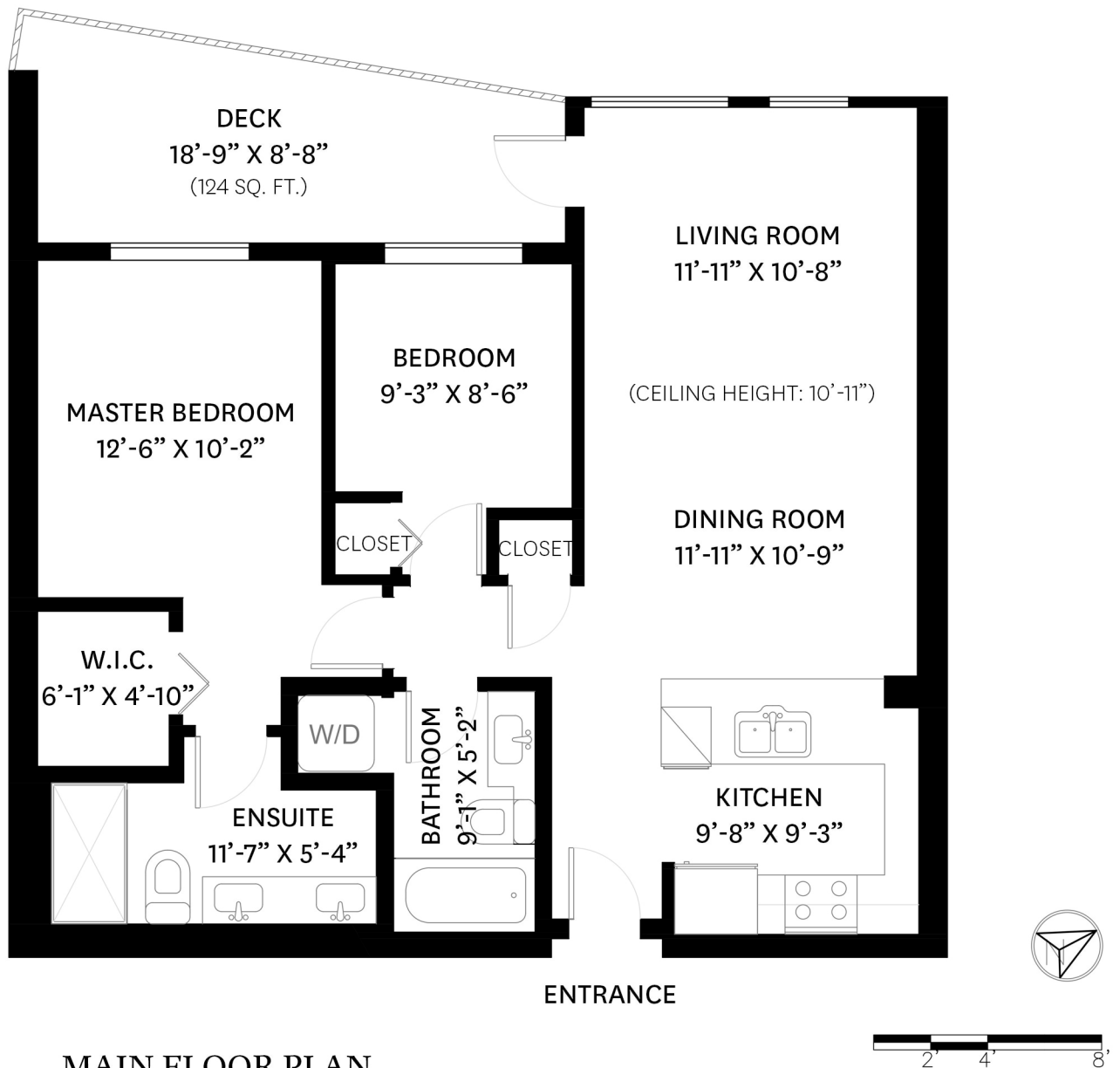
MAIN FLOOR PLAN Ceiling Height: 9'-0"
