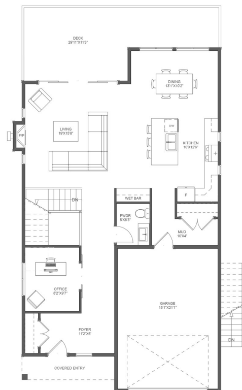
○ MAIN FLOOR PLAN (9' CEILING) MAIN FLOOR AREA: 1,040.93 Sq Ft GARAGE FLOOR AREA: 352.00 Sq Ft
