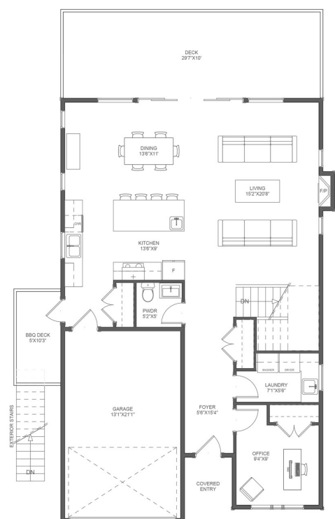
MAIN FLOOR PLAN (9' CEILING) MAIN FLOOR AREA: 1,050.41 Sq Ft GARAGE FLOOR AREA: 307.57 Sq Ft
